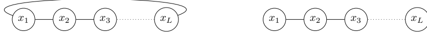
Figure 3.2: Bravais lattices of periodic (Born-von Karman) bounds (left), and terminal bounds (right). The lines between nodes indicate the hopping terms in the Hamiltonian. For the uniform chain, all edges of the graph have the same amplitude and are thus unmarked.
